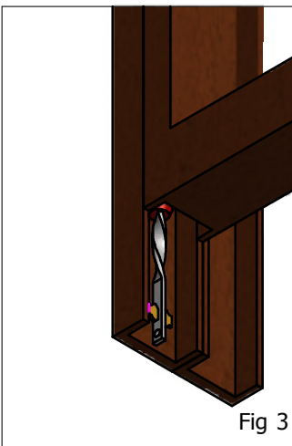
Fig 3: Raise the sash and support its weight on a suitable strut. Unhook and clear the spiral rod of its fixing bracket. Lower the rod by up to a maximum of 50mm. Should the rod extend out of the balance by more than 50mm, gently push the rod back into the balance, allowing it to rotate freely.
