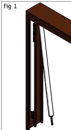
Fig 1: Load balances into outer frame before installing sashes, then load the sash into the frame. If window is already installed, see Fig 1A.
