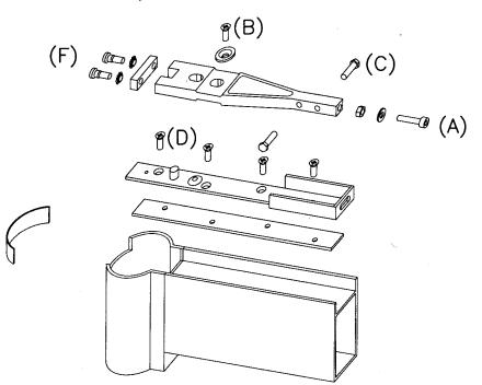
Prepare the top rail of the door as detailed, ensuring that the internal faces of the stile and top rail have been cut away to enable the closer spindle to be engaged during door hanging.
