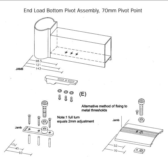
Prepare the bottom rail of the door to accommodate the pivot shoe with 2No.drilled and tapped M6 holes at 98.5mm and 143mm centres.
