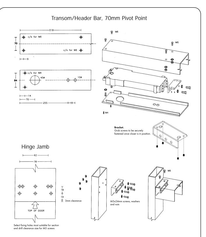
Prepare transom/header bar and cover plate to accept closer as detailed below. Fit jamb bracket to jamb with the 5 No. M5x24mm screws, washers and nuts.
