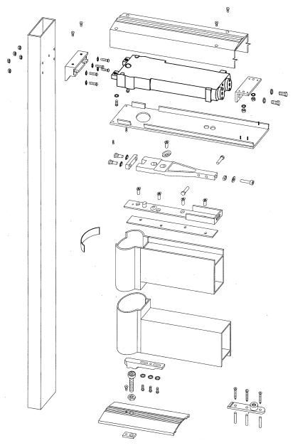
**NOTE:** The thread of all fixings should be applied with Loctite 222 or similar and securely fastened.
